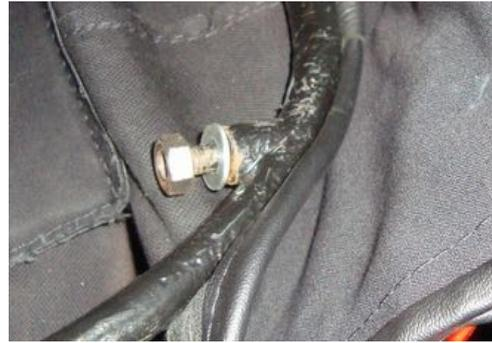
*The bolt and nut (originally a winged nut) for fixing the hood at the windscreen.*
