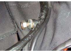
The bolt and nut (originally a winged nut) for fixing the hood at the windscreen.
