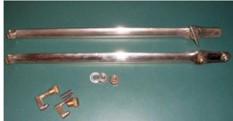
The two columns which are attached at the windscreen, the two nuts for fixing the frame at the columns, and two stabilizers for the frame.
